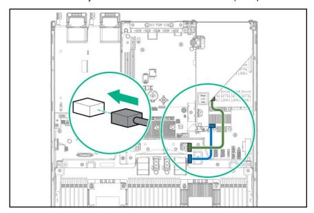
PCI slot-based Smart Array controller with x8 connector (Group A SAS cables)
