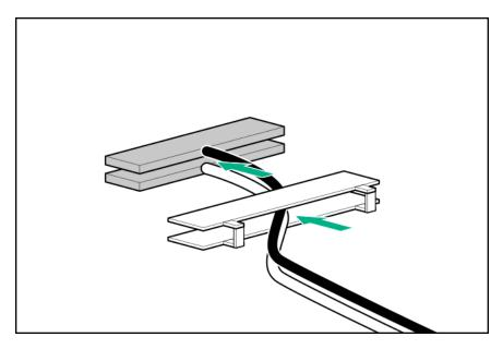
Open the cable latch door, connect the auxiliary card cables to the adapter ports so that the golden side of the cable connector is on the top, and then close the cable latch door.
