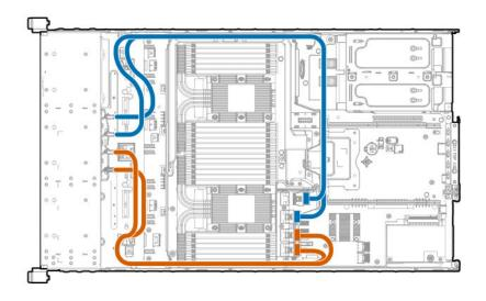
Two-bay NVMe/Six-bay SFF HDD drive cages installed in boxes 1–3
