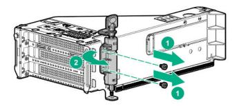
Install the additional fastener supplied with the option kit onto the riser cage.
