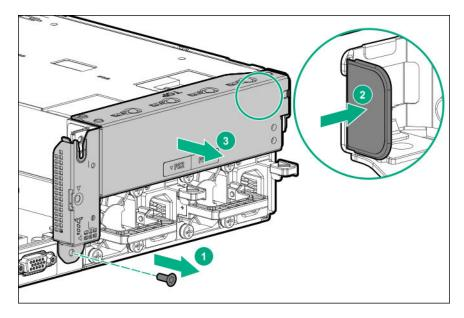
7. Install the power supply cage.
