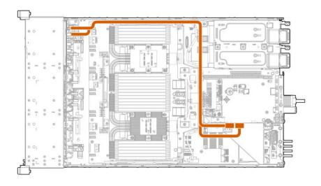
Connected to the secondary PCle riser board
