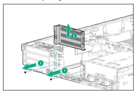
6. When installing the secondary PCIe riser cage for the first time, remove the fastener from the riser cage.
