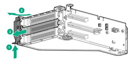
Install the expansion board into the PCI riser cage.
