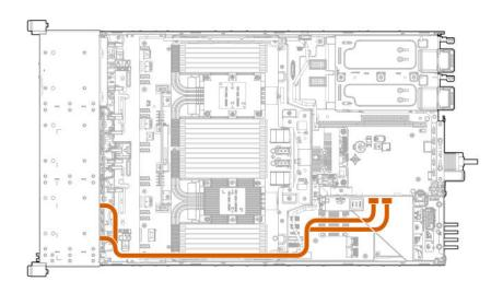
Connected to the secondary PCle riser board
