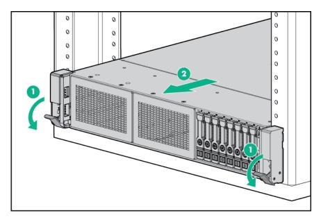
**3.** After performing the installation or maintenance procedure, slide the server back into the rack, and then press the server firmly into the rack to secure it in place.
