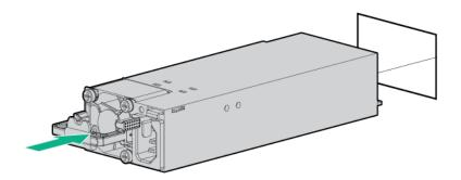
**4.** Connect the power cord to the power supply.
