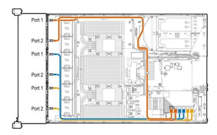
From the drive cage backplane to the controller in the secondary PCIe riser cage
