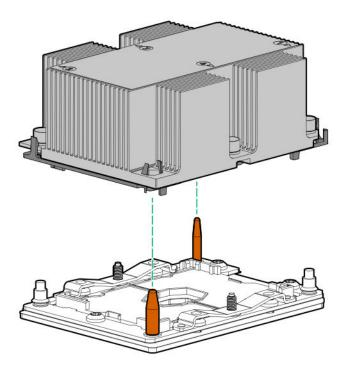
**CAUTION:** Be sure to tighten each heatsink nut fully in the order indicated. Otherwise, boot failure or intermittent shutdowns might occur.
