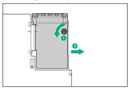
Install the FlexibleLOM adapter.
