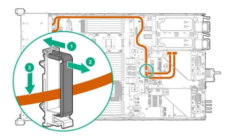
Connected to the tertiary PCIe riser board
