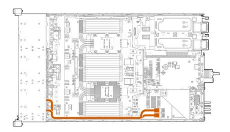
Connected to an HPE Smart Array controller
