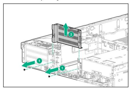
**6.** Remove the power cage blank.
