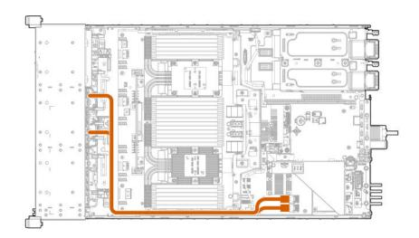
Connected to the Smart Array controller
