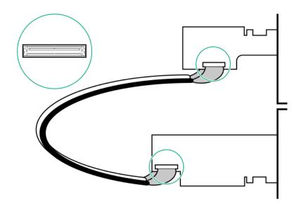
**13.** Install the adapter and auxiliary cards into x16 slots.
