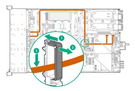
Connected to the tertiary PCIe riser board
