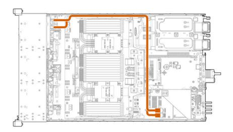
Connected to the HPE P816i-a Smart Array controller
