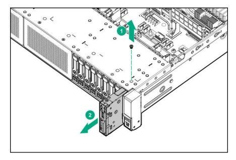
**8.** Route the cable through the opening in the front of the server, and then install the SID power switch module. Secure the module using the existing screw.
