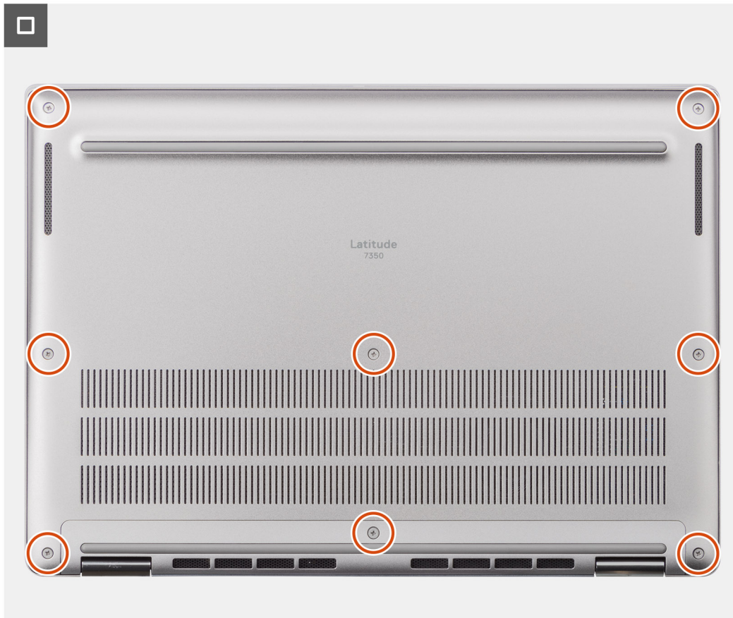
Figure 20. Installing the base cover
