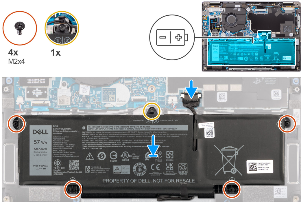
Figure 32. Installing the 3-cell battery
