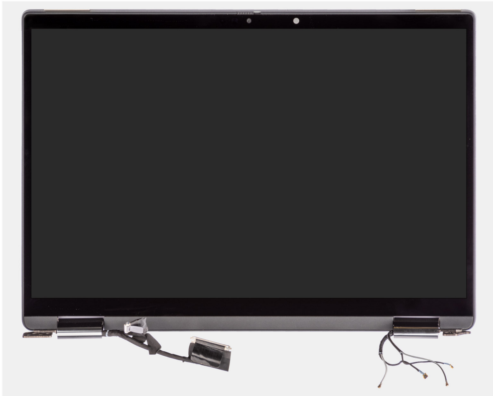
Figure 43. Display assembly without WWAN-antenna cables
