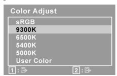
**sRGB**—sRGB is quickly becoming the industry standard for color management, with support being included in many of the latest applications. Enabling this setting allows the LCD display to more accurately display colors the way they were originally intended. Enabling the sRGB setting will cause the Contrast and Brightness adjustments to be disabled.
