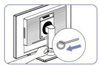
You can remove the fixing pin and adjust the stand now.
