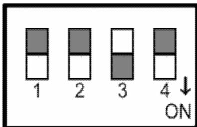
**OFF:** If Pin 3 is in the OFF position, the 110VDSLEXT / GB / EU will operate in Symmetric mode, with both downstream and upstream transmissions operating on the G.997 band plan.
