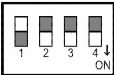
**OFF:** If Pin 1 is in the OFF position, the 110VDSLEXT / GB / EU will operate in Central Office (CO) mode.
