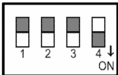
**OFF:** If Pin 4 is in the OFF position, the 110VDSLEXT / GB / EU will operate with a SNR ratio up to 9 dB.
