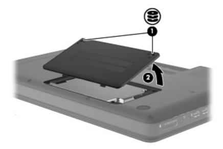
Remove the hard drive screws (1), and then lift the hard drive slightly (2).
