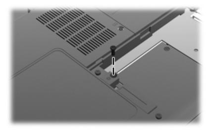
11. Align the tabs (1) on the hard drive cover with the notches on the computer, close the hard drive cover (2), and tighten the hard drive screws (3).
