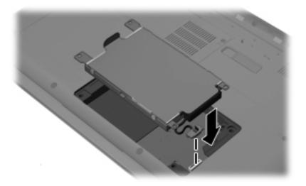
2. Snap the hard drive into place (1), and then replace the hard drive screws (2).
