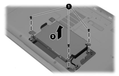
**10.** Disconnect the hard drive cable, and then lift the hard drive away from the computer.
