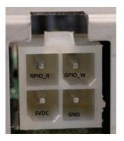
Mating connectors can be found at: <a href="https://www.molex.com">www.molex.com</a> Mates with the 5557 Mini-Fit Jr. Receptacle Housing
