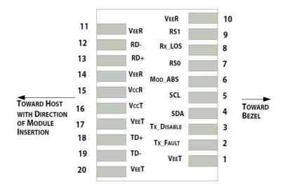
Pin-out of connector Block on Host board
