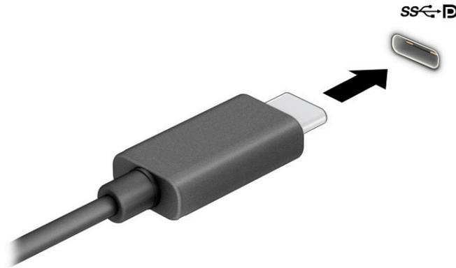
2. Connect the other end of the cable to the external DisplayPort device.
