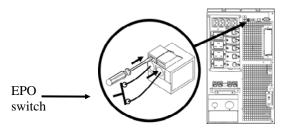
Both Class 2 and SELV circuits must be isolated from all primary circuitry. Do not connect any circuit to the EPO terminal block unless it can be confirmed that the circuit is Class 2 or SELV. If circuit standard cannot be confirmed, use a contact closure switch.
