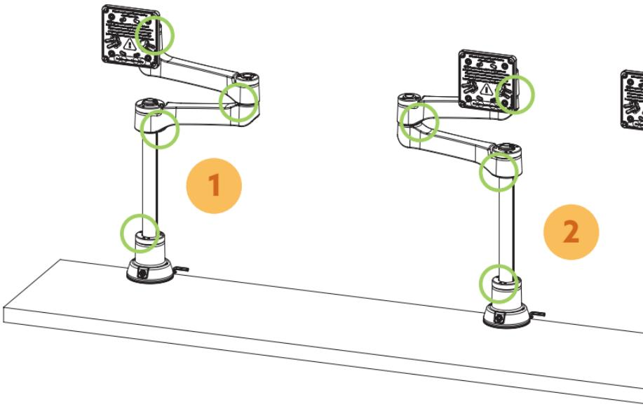
\* **Smart Stop™:** At the bottom of the ring there is a small arrow. This arrow indicates where the Smart Stop™ is, i.e. where the arm stops rotating. It is important to have the arrow on the correct side (left or right), so that the arm stops rotating and for example does not bump into an acoustic screen (see p. 10 & 11 for setup).
