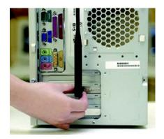
Figure 3-5: Positioning the Antenna
