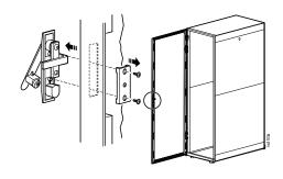
Disconnect the ground wire, and any other connections. Remove the door from the frame.
