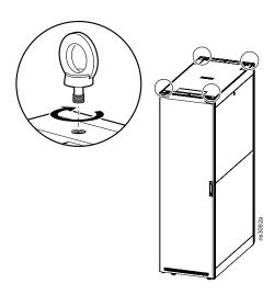
Assure a straight-line pull on the lifting eye bolts when lifting the Easy Rack.
