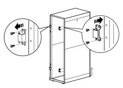
Rotate the door. Remove the hinges from the door, and install them to the alternate hole location. The hinges on the door should now align with the hinges on the rack.
