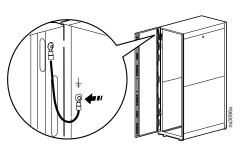
The hinges come apart by lifting the door up and away from the rack.
