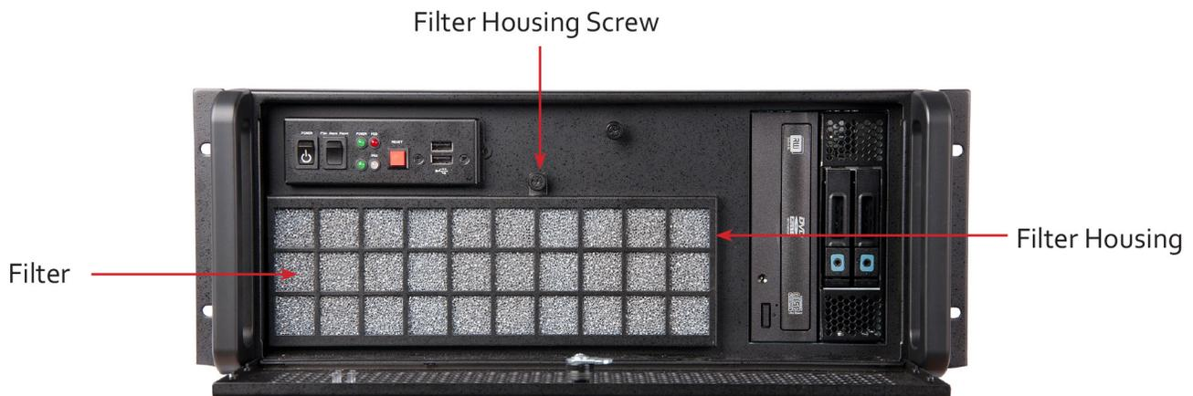
Figure 6-1. Filter location on the VWP-2090 or VWP-2110.
