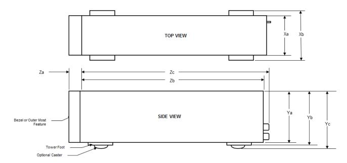
Figure 1. Chassis dimensions
