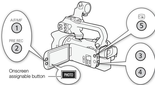
**1 Physical buttons:** Press the MENU button and, while holding it pressed down, press the assignable button whose function you wish to change.
