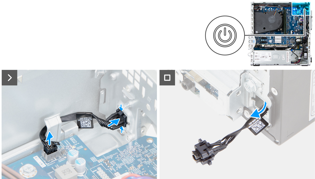
Figure 43. Removing the power button
