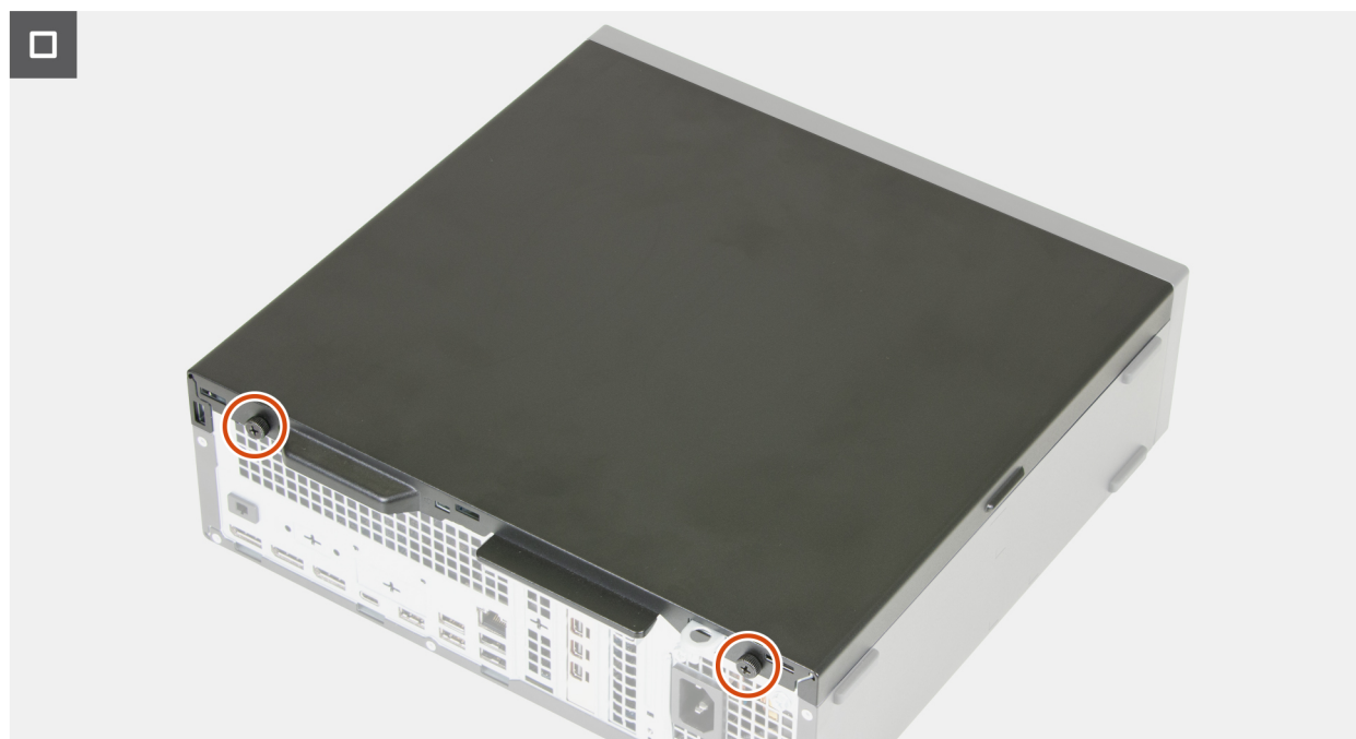
Figure 9. Installing the side cover
