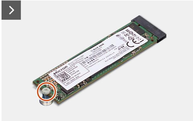
Figure 24. Removing the M.2 2280 solid state drive
