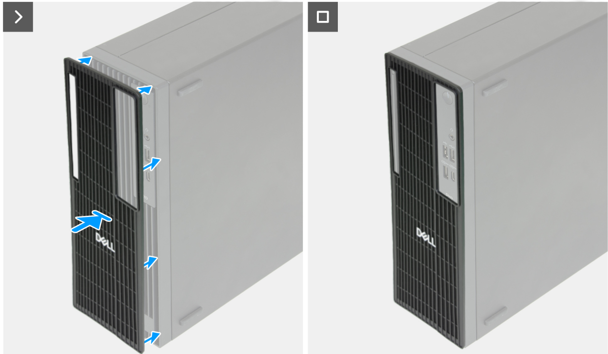
Figure 15. Installing the dust filter
