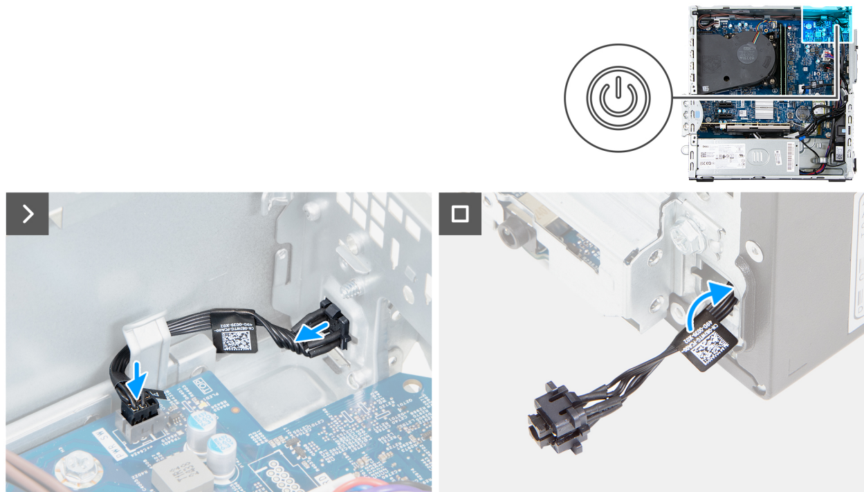
Figure 44. Installing the power button
