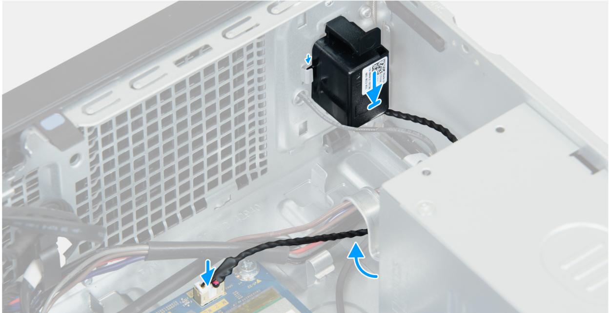
Figure 19. Installing the internal speaker
