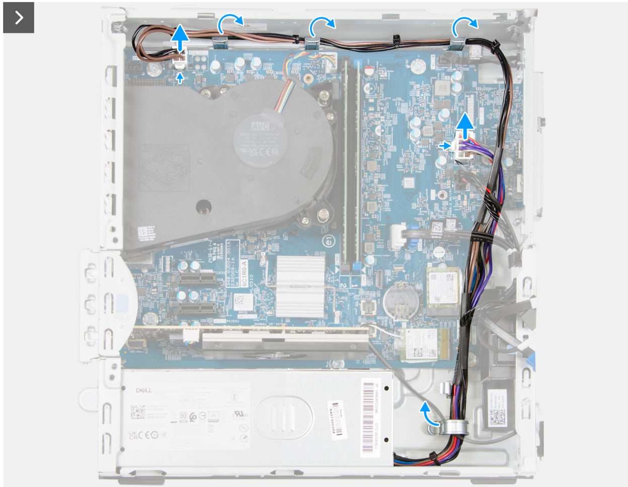
Figure 47. Removing the power-supply unit
