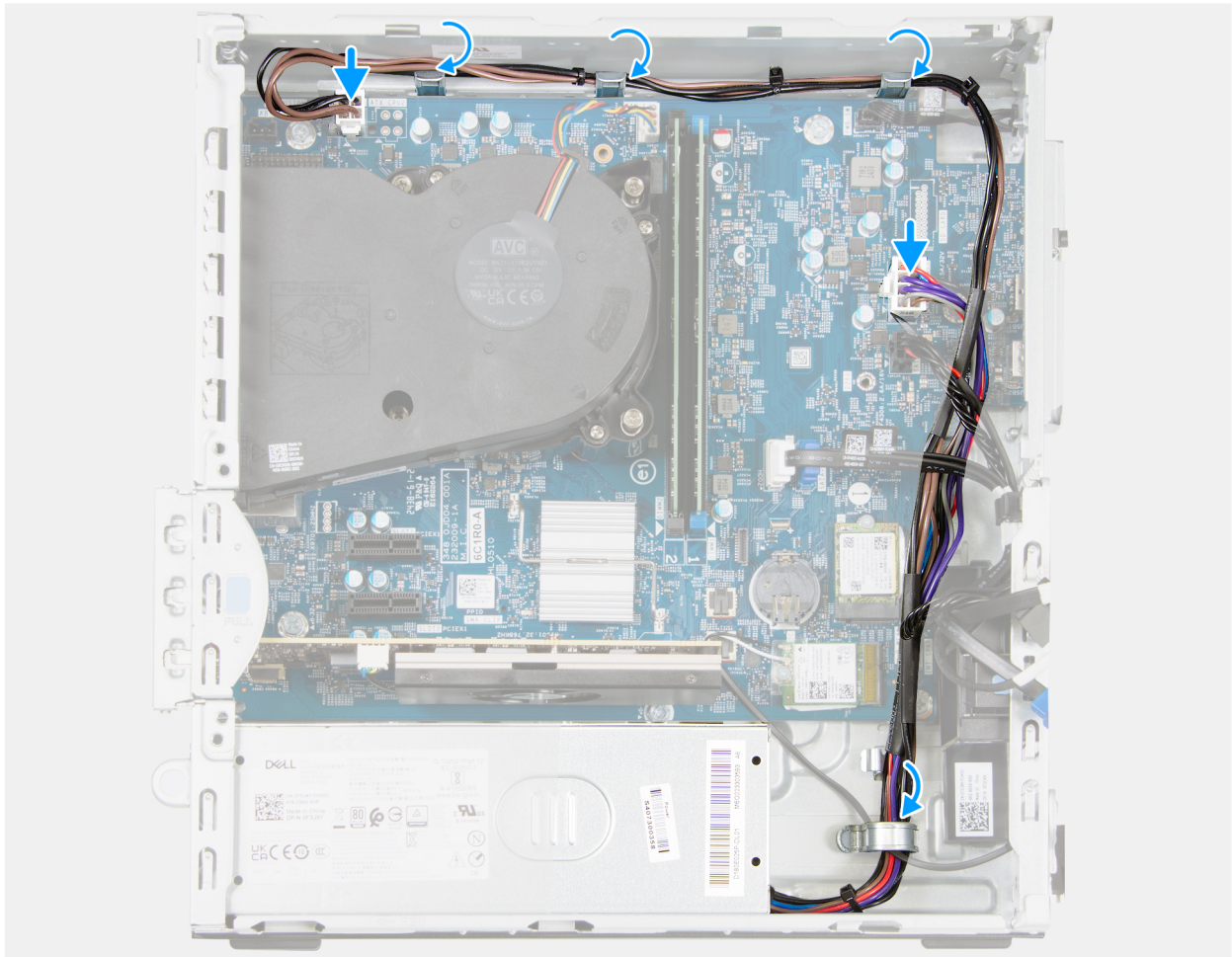
Figure 50. Installing the power-supply unit
