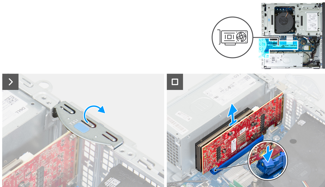
Figure 27. Removing the graphics card
