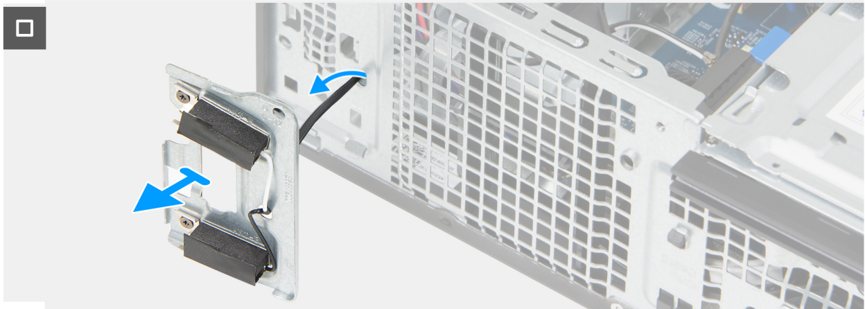
Figure 45. Removing the antenna modules
