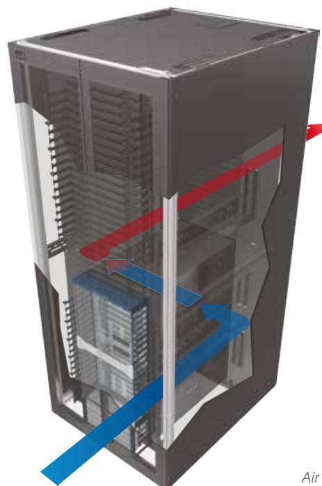
*Air flow in switch rack for switches equipped with lateral cooling.*
