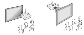
Make sure you select the correct **Projection** option in the projector's **Settings** menu according to the installation method being used.
