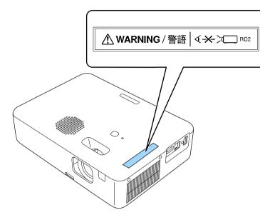
As with any bright source, do not stare into the beam, RG2 IEC/EN 62471-5:2015.
