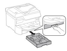
Slide the side edge guides all the way out and set the front edge guide to the paper size you are using.
