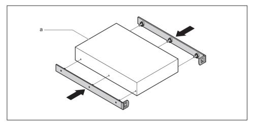
Fasten the EasyChange rails to the side of the drive or adapter by inserting each pin of the EasyChange rail in the corresponding holes on the drive. In doing so, make sure that the ports on the drive are located at the rear as shown (a).
