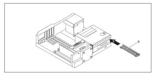
Slide the drive plate (a) into the upper bay (5) again as shown, until it engages.
