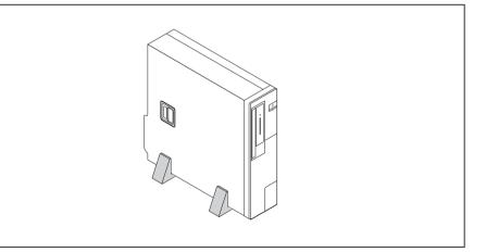
Stand the device on the feet as shown.
