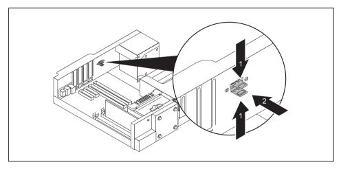
Keep the clips (1) pressed and push the sheet metal plate out of the casing from the inside (2).
