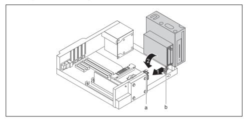
Gently press the upright bracket (b) of the drive cage in the direction of the arrow (1) until you can move the drive cage.
