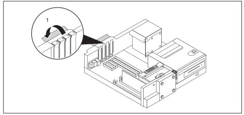
▶ Fold out the board retaining mechanism (1).
