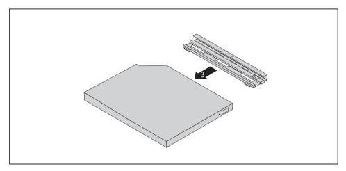
• Secure the drive plate on the slimline drive as shown (3).
