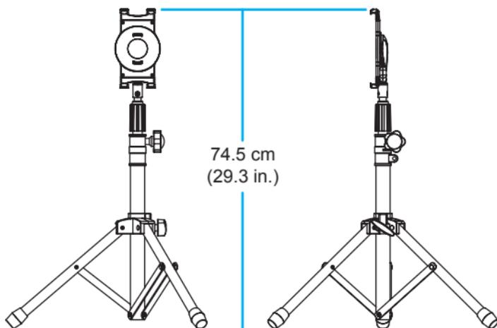
Dimensions of tripod when it's extended and the tablet holder is attached
