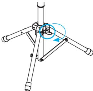
3. Turn the hand screw on the pole of the tripod to the left to loosen it.
