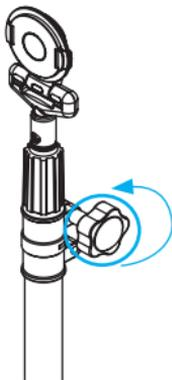
4. Move the tripod pole up or down to your desired height and turn the hand screw on the tripod to the right to tighten it.
