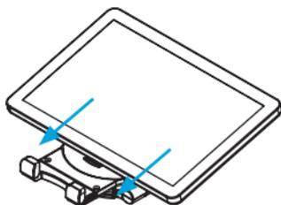
2. Pull out the other retractable bracket to open it up and place the bracket claw over the other side of the tablet. Gently release the bracket.
