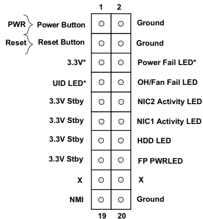
Figure 3-1. JF1: Control Panel Pins
