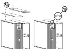
2. Install the tie bracket securing the UPS and external battery pack (screws included).
