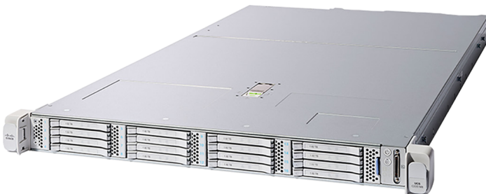
Figure 1. Cisco Compute Hyperconverged with vSAN HCIVS220C M8 All-NVMe Server
