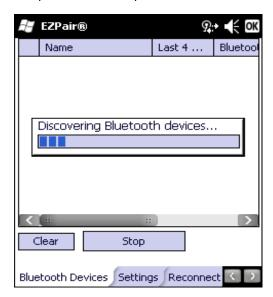
2. Tap the Stop Button at any time to end the Discover and Query for Unique Identifier functions. The Bluetooth Device List is displayed.
