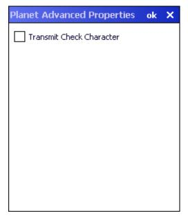
Transmit Check Character – When enabled, transmit the check character. Default is enabled.
