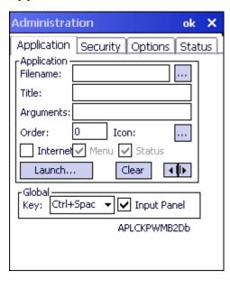
Use the Application tab options to select the applications to launch when the device boots up in End user Mode.
