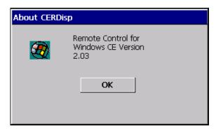
6. Click the OK button to dismiss the About CERDisp dialog box on the MX7 Tecton desktop by clicking the OK button in the HSM Connect window on the PC desktop. The dialog box automatically times out and disappears after approximately 20 seconds.
