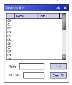
Note: After adding, changing and removing items from the Custom IDs list, tap the ok button to save changes and return to the Barcode panel.
