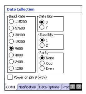
Integrated laser scanner default values are 9600 Baud, 8 data bits, 1 stop bit and No parity.
