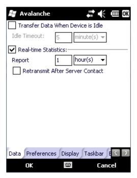
The Data tab controls when data is transferred between the MX7 Tecton and the Mobile Device Server.
