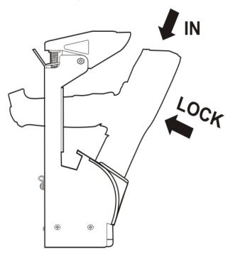
Do not slam the MX7 Tecton into the cradle pocket. Damage to the cradle and MX7 Tecton components may occur. If the vehicle cradle or MX7 Tecton is damaged, it must be removed from service and repaired before placing it into service again.
