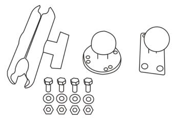
Mount the cradle U-bracket to the upper RAM ball assembly with the bolts, washers and nuts supplied by Honeywell.
