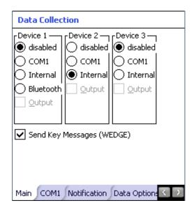
Panel showing options for Symbol or Honeywell scan engine
