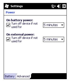
Select the inactivity timeout period before the MX7 Tecton goes into Suspend mode. The settings on this panel are for the suspend timers only.
