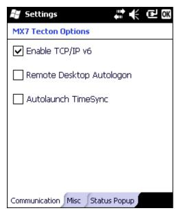
By default, TCP/IP version 6 is enabled on the MX7 Tecton. Tap to uncheck this check box to disable TCP/IP version 6. By default, Remote Desktop Autologin is disabled. Tap this check box to enable Remote Desktop Autologin. Autolaunch TimeSync enables time synchronization when the MX7 Tecton boots.
