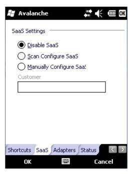
Use to configure the Enabler to connect with Avalanche on Demand. This is a Software-as-a-Service version of Avalanche. Using either of the SaaS configuration options below assumes the user has registered with Wavelink.
