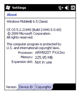
This screen displays information on the installed operating system and the hardware. Note that Windows Mobile is based on a Windows CE engine. The underlying version of Windows CE is displayed here.
