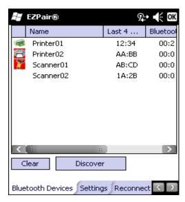
The discovered paired devices may or may not be identified with an icon. Discovered devices without an icon can be paired as a Serial device, Scanner or a Printer. The Bluetooth panel assigns an icon to the device name.
