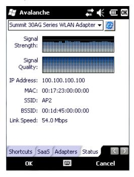
Link speed indicates the speed at which the signal is being sent from the adapter to the MX7 Tecton. Speed is dependent on signal strength.
