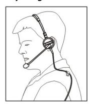
Do not twist the microphone boom when adjusting the microphone. The microphone should be adjusted to be about two finger widths from your mouth.
