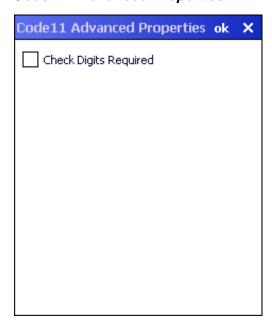
**Check Digits Required** – When enabled, only bar codes with two check digits are decoded. The default is disabled.
