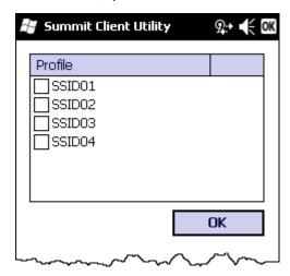
The Auto Profile selection screen displays all currently configured profiles. Tap on the check box for any profiles that are to be included in Auto Profile selection then tap ok to save.
