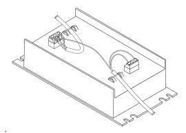
Note: The input block has V<sub>IN+</sub>, V<sub>IN-</sub> and GND terminals. The output block has V<sub>O+</sub> and V<sub>O-</sub> terminals.
