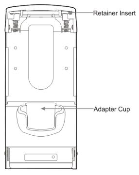
The MX7 Tecton cradle charging pocket, without a cradle adapter cup and top adapter, is designed for an MX7 Tecton with a rubber boot (MX7490BOOT or MX7491BOOT) enclosing/protecting the MX7 Tecton.
