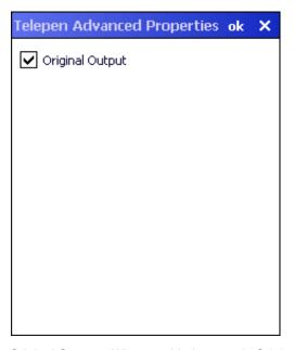
Original Output - When enabled, output is Original Telepen. When disabled, output is AIM. Default is enabled.
