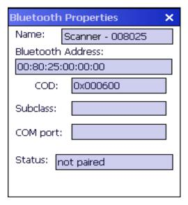
Data on the Bluetooth Properties panel cannot be changed by the user. The data displayed is the result of the device Query performed during the Discovery process.
