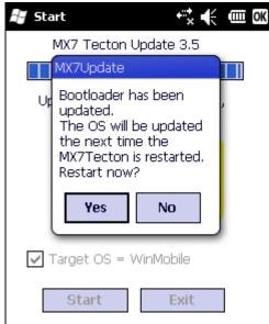
When the bootloader process is complete, tap the Yes button to reboot to complete the update process. Tap the No button and the update is not complete.
