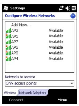
2. If the desired network is not displayed, tap **Add New**. If the desired network is displayed in the list, tap the network name.
