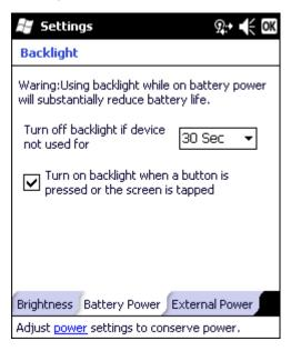
When the MX7 Tecton is on battery power and the backlight timer expires, the display and the backlights for the display and keypad are turned off. Adjust the settings and tap OK to save the changes. The changes take effect immediately.
