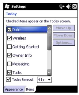
The **Today timeout** timer refers to the "return to Today screen" function. When the device is placed in Suspend, and the timer expires, a return from Suspend displays the Today screen, not the application in focus when the MX7 Tecton was placed in Suspend. The application in focus, which is running in the background, will need to be selected again.
