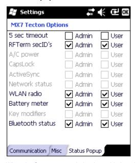
When the Status popup window is enabled, and displayed, it is placed on top of the window in focus and hides any data beneath it.
