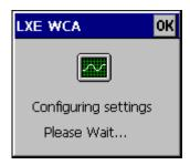
Once configured, the MX7 Tecton is warmbooted. After it reconnects to the wireless network and the Mobile Device Server, any software updates and additional configuration data are downloaded.
