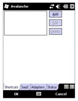
Configure shortcuts to other applications on the MX7 Tecton. Shortcuts are viewed and activated in the Programs panel. This limits the user's access to certain applications when the Enabler is controlling the mobile device display.
