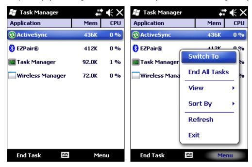
Tapping on the column headings at the top of the screen sorts the tasks by the contents of that column. Tapping the same heading a second time reverses the sort order of that column.
