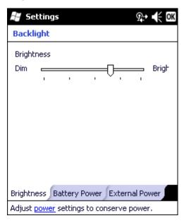
Slide the marker left and right to select the desired keypad and display brightness level. Adjust the settings and tap OK to save the changes. The changes take effect immediately
