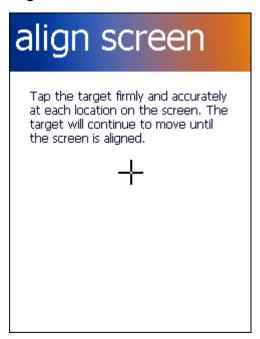
Tap the Align Screen button. The align screen opens and displays a large cross-hair in the middle of the screen. Tap the middle of the cross-hair as it moves around the screen. When the process is complete, the General screen is displayed. Tap ok and the changes are saved. The new alignment is in effect immediately.
