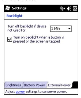
When the MX7 Tecton is on external power and the backlight timer expires, the display and the backlights for the display and keypad are turned off. Adjust the settings and tap OK to save the changes. The changes take effect immediately.
