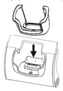
The adapter cup is installed facing in one direction.
