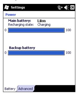
Battery power is displayed for both the main and internal Super-cap batteries (backup battery).
