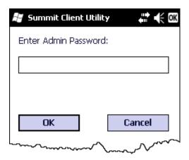
Enter the Admin password (the default password is SUMMIT and is case sensitive) and tap OK. If the password is incorrect, an error message is displayed.
