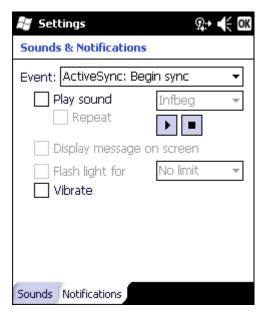
The Event box lists several events that can have an associated notification. The notification, depending on the event selected, may consist of playing a sound, displaying a screen message, flashing a light or triggering the vibration motor.
