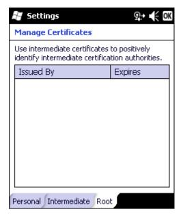
This panel lists any installed Root certificates. Root certificates are used to authenticate certificates received from other hosts.
