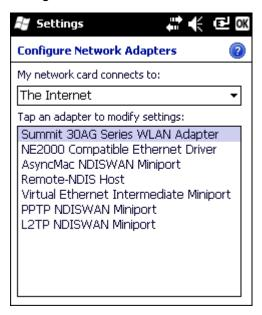
To configure a network card, tap on the adapter name and enter the IP address (or select Use server assigned IP address) and the name server addresses.
