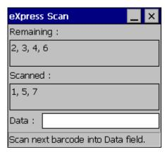
7. The remaining bar codes may be scanned in any order. After a bar code is scanned, the bar code is removed from the "Remaining:" list and placed in the "Scanned:" list.
