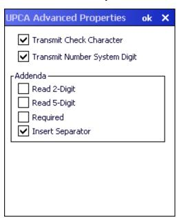
Transmit Check Character – When enabled, transmit the check character. Default is enabled
