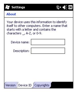
The device name and description can be changed by the user. Enter the name and description using either the keypad or the Input Panel and tap ok to save the changes. The changes take effect immediately.
