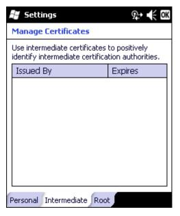
This panel lists any installed Intermediate certificates. Intermediate certificates are used to help authenticate certificates received from other hosts.
