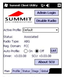
The Main tab displays information about the wireless client device including:
