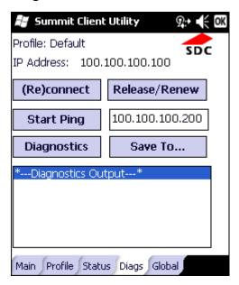
The Diags screen can be used for troubleshooting network traffic and radio connectivity issues.
