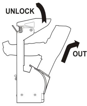
2. Pull the MX7 Tecton up and out of the vehicle cradle pocket, disconnecting the MX7 Tecton from the charge/communication port at the base of the docking bay. The Docked LED turns off.
