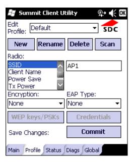
When logged in as an Admin, see Admin Login (page 11-6), use the Profile tab to manage profiles. When not logged in as an Admin, the parameters can be viewed, and cannot be changed. The buttons on this tab are dimmed if the user is not logged in as Admin. The Profile tab was previously labeled Config.
