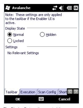
The Display State options control the appearance of the taskbar while using the Enabler interface.
