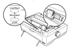
5. Press the Pause button to exit the Micro Adjust mode.
