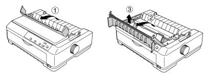
2. Remove the paper tension unit by pressing up the tabs on each side and pulling it up.
