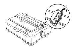
4. Slide the left sprocket approximately 0.5 inch (12 mm) from the far left position and push the blue lever back to lock it in place. Then slide the right sprocket to match the width of your paper, but do not lock it.
