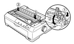
8. To replace the printer cover, insert the front tabs into the slots on the printer and lower the cover into place. Then push it down until it clicks.
