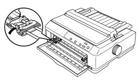
4. Slide the left sprocket approximately 0.5 inch (12 mm) from the far left position and pull the blue lever forward to lock it in place. Then slide the right sprocket to match the width of your paper, but do not lock it.
