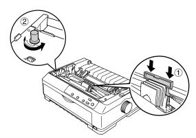
7. Reinstall the paper tension unit by lowering it onto the printer's mounting pegs. Then press down on both ends until it clicks into place.
