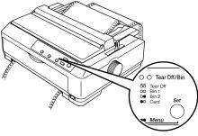
3. Open the paper guide cover, then press the LF/FF ♣ button to feed paper backward, or press the Load/Eject ♠ button to feed paper forward, until the paper perforation is aligned with the tear-off edge of the printer cover.
