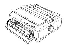
2. Set the paper release lever to the front push tractor position. Also set the paper-thickness lever to the proper position for your paper's thickness. See "Adjusting the Paper-Thickness Setting" on page 18 for instructions.
