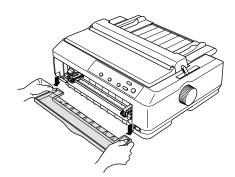
6. Make sure your paper has a clean, straight edge. Then open both sprocket covers and fit the first four holes of the paper, with printable side up, over the tractor pins.
