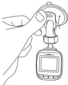
4) When finding the best mounting location on the windshield, steadily place it onto the windshield and lock it into place.
