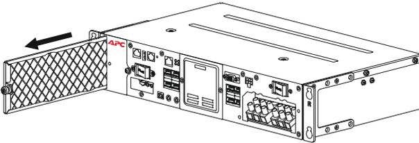
3. Slide the replacement filter into the chassis.
