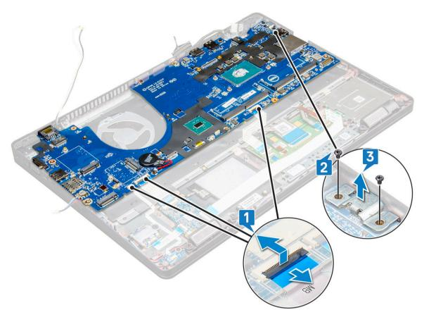
Remove the M2.0x3.0 screws (3) and lift the system board away from the computer [1, 2].
