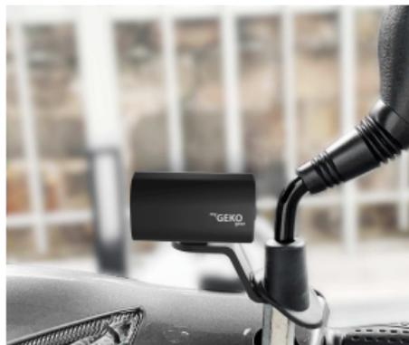
Note: Regardless of whether the camera is installed on the left or right side, the myGEKOGear logo on the snap mount must always be upright and face out, with the LED indicator lights always facing up. Below are installation examples for reference.
