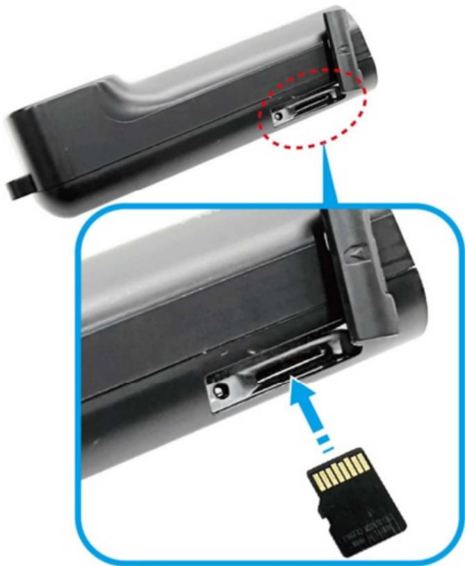
The slot cover must be tightly sealed to prevent moisture from entering, causing the lens to fog. Insert the lower edge of the slot cover, then press the top edge and sides of the slot cover to create a good seal. See below.
