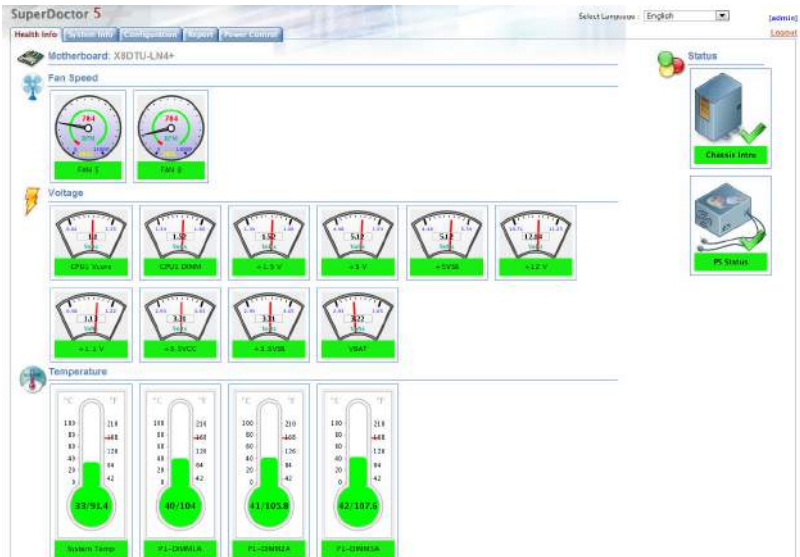
Figure 5-7. SuperDoctor 5 Interface Display Screen (Health Information)
