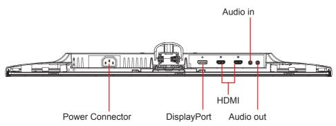
3.A. Please do not connect the DisplayPort out on the monitor to the DisplayPort or mini DP connector on the computer. DisplayPort out is used for daisy chain connection (Explained in section D)
