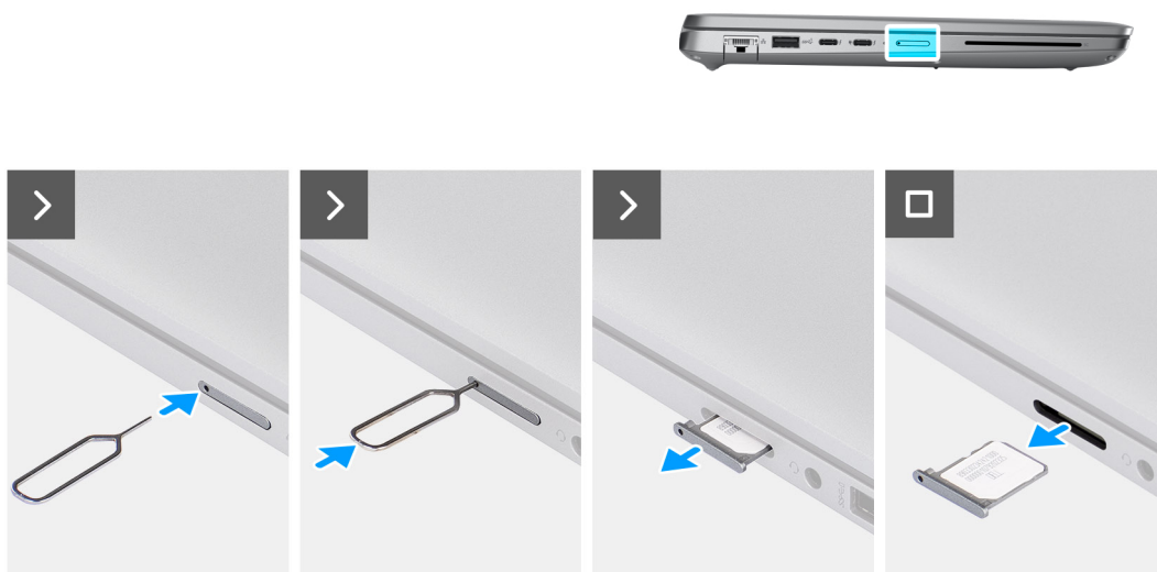
Figure 2. Removing the SIM card tray
