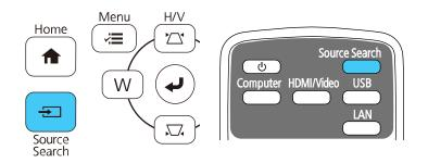
• Press the button for the source you want on the remote control. If there is more than one port for that source, press the button again to cycle through the sources.
