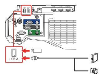
**Note:** Do not connect a USB hub or a USB cable longer than 10 feet (3 m), or the device may not operate correctly.
