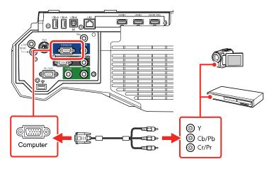
3. Tighten the screws on the VGA connector.
