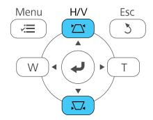
3. Press a keystone button on the projector's control panel to adjust the image shape.
