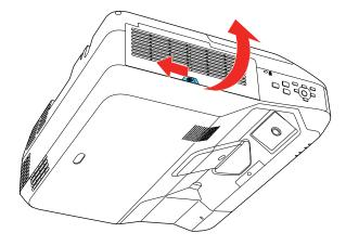
3. Raise or lower the focus lever to sharpen the image.
