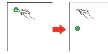
Note: For the most accurate calibration, make sure you touch the center of the circle.
