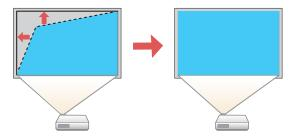
**Note:** Use the adjustment dials on the wall mount to correct the screen image before using any other digital correction methods.
