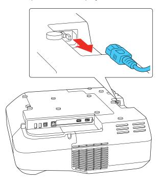
**Caution:** To avoid damaging the projector or laser, never unplug the power cord when the Status light is on or flashing.
