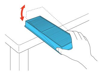
**Caution:** Do not use excessive force when tapping the air filter, or it may crack and become unusable. Do not rinse the air filter in water, or use any detergent or solvent to clean it. Do not use
