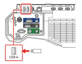
**Note:** Connect the flash drive directly to the projector. Do not use a hub or your settings may not be saved correctly.
