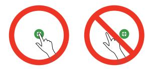
**Note:** Make sure you are not blocking the signal between your finger and the interactive receiver (next to the projection window on the projector).
