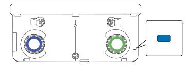
**Note:** If the blue light does not turn on, press the **Menu** button on the remote control and make sure the **Extended > Easy Interactive Function > Touch Unit Setup > Power** setting is set to **On**.
