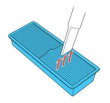
Note: If dust is difficult to remove or the air filter is damaged, replace the air filter.
