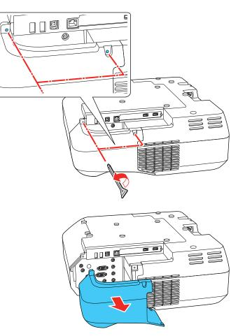
To attach the cable cover, slide it into position and tighten the screws with a screwdriver. **Parent topic:** Setting Up the Projector
