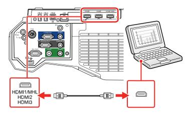
**Note:** The projector converts the digital audio signal sent from your computer into a mono analog signal for the internal speaker or a stereo analog signal if you are connecting to external speakers. (Make sure the HDMI audio playback device on your computer's audio settings is set to **EPSON PJ**.)
