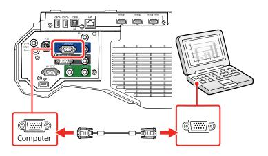
4. Tighten the screws on the VGA connector.
