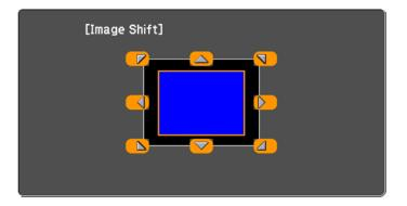
3. Use the arrow buttons on the projector or remote control to adjust the image position.
