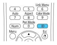
5. Press the ID button on the remote control to check if the ID-setting process worked.
