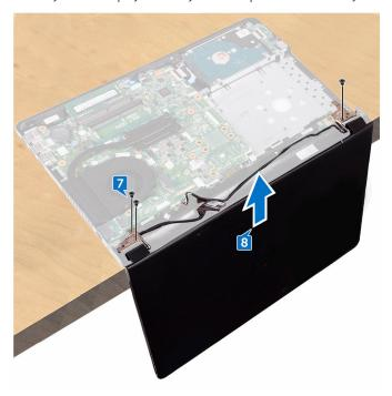
Carefully place the display assembly on a clean and flat surface.
