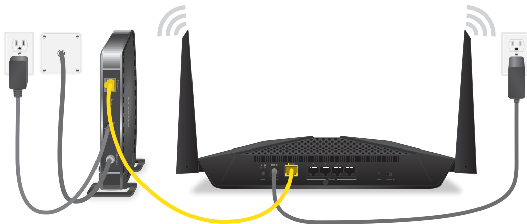
Figure 6. Cable your router
