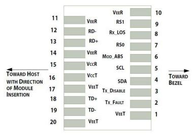
Pin-out of connector Block on Host board
