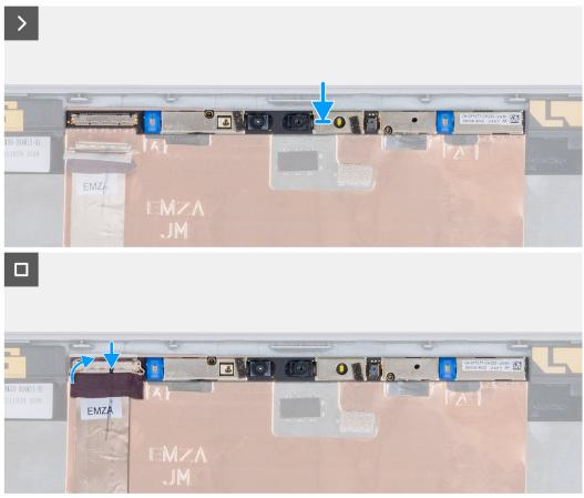
Figure 3. Installing the camera module
