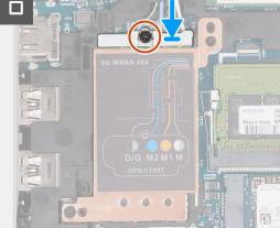
1. Connect the antenna cables to the 5G WWAN card.
