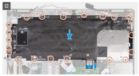
1. Align and place the keyboard on the keyboard bracket.
