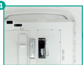
4 Lift the SSD off the compartment.
