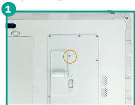
1 Loosen the screw on the back side of the tablet.
