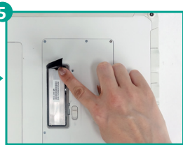
5 Fit another SSD into place.
