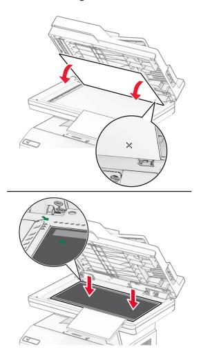
Close the scanner cover to attach the new scanner glass pad.
