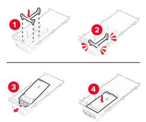
Secure the ISP in place, and then attach the ISP extended cable.
