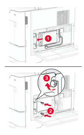
Attach the hard disk interface cable to the controller board.
