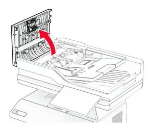
2 Remove the used ADF pick roller.
