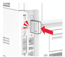
**9** Insert the fax card, and then install the screws.
