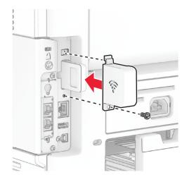
11 Close the controller board access cover, and then install the screw.
