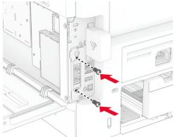
**10** Attach the wireless print server cover, and then install the screw.
