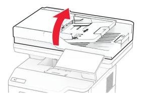
Remove the used scanner glass pad.
