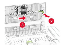
Remove the used ADF separator roller.
