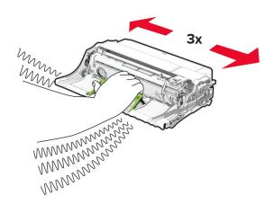
**Warning—Potential Damage:** Do not expose the imaging unit to direct light for more than 10 minutes. Extended exposure to light may cause print quality problems.
