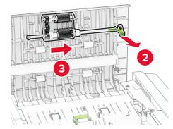
**3** Remove the ADF separator roller.
