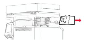
**6** Remove the used power supply.
