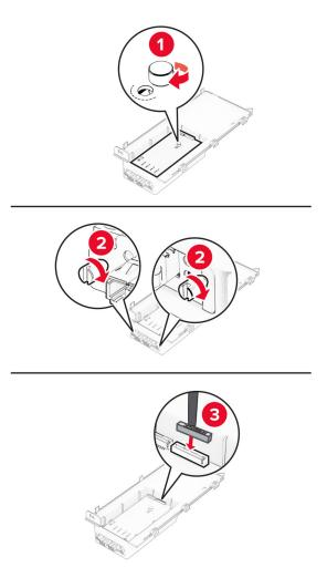
Using a flat-head screwdriver, remove the controller board access cover.
