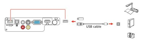
If you connect a digital camera, USB flash drive, or USB storage device, you can use the projector's PC Free feature. You can also connect other Epson document cameras to the projector. See the online *User's Guide* for details.
