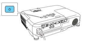
**Note:** To shut down the projector, press the  $\bigcirc$  power button twice, then unplug it. You don't have to wait for the projector to cool down.
