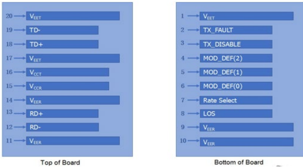
Pin-out of connector Block on Host board
