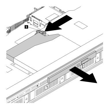
Figure 87. Removing the optical drive
