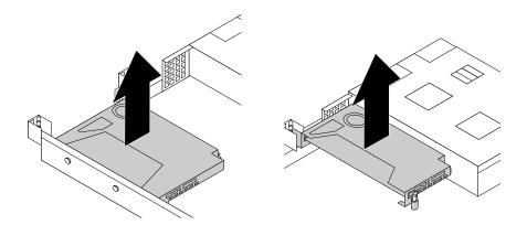
Figure 96. Removing the riser card assembly
