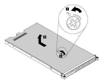
Figure 19. Removing the server cover
