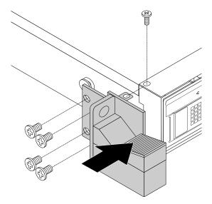
Figure 21. Installing the rack handles
