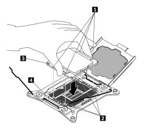
Figure 59. Installing the microprocessor
