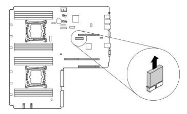
Figure 31. Removing the TPM
