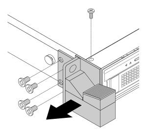
Figure 20. Removing the rack handles
