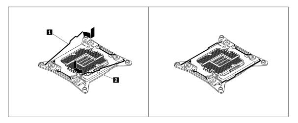
Figure 105. Securing the microprocessor retainer
