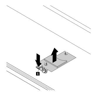
Figure 37. Removing the SD module
