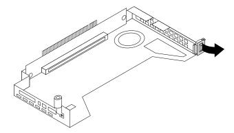
Figure 42. Opening the PCIe card latch
