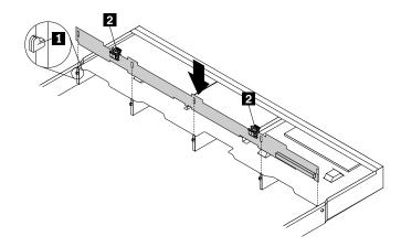
Figure 91. Installing the hot-swap hard-disk-drive backplane
