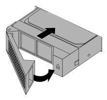
Figure 75. Installing the hot-swap hard disk drive
