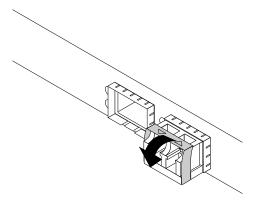
Figure 50. Pivoting the optical module handle
