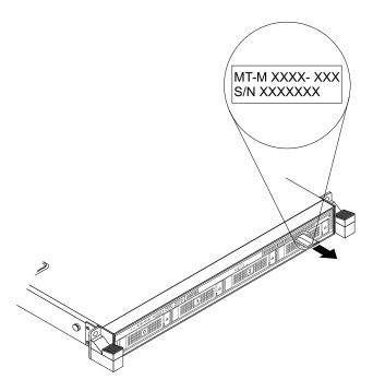
Figure 1. Label on server models with 3.5-inch-drive bays
