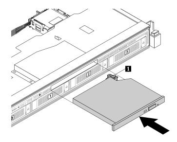
Figure 88. Installing the optical drive
