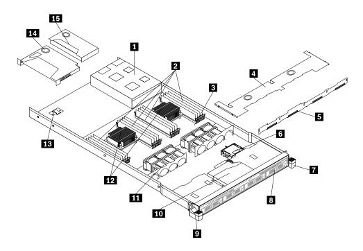
Figure 7. Components of server models with 3.5-inch drives
