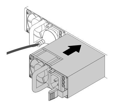
Figure 70. Installing a hot-swap redundant power supply
