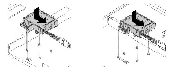
Figure 39. Installing the ThinkServer RAID Super Capacitor Module
