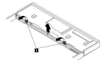
Figure 90. Removing the hot-swap hard-disk-drive backplane
