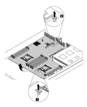
Figure 102. Removing the system board
