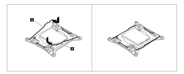
Figure 67. Securing the microprocessor in the socket
