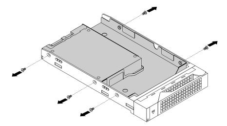
Figure 84. Removing the screws that secure the solid-state drive and the drive adapter
