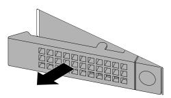
Figure 77. Removing the dummy hard-disk-drive tray
