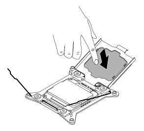
Figure 60. Removing the microprocessor socket cover
