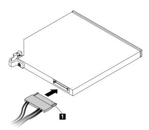
Figure 89. Connecting the connector 1 to the rear of the optical drive
