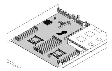
Figure 103. Installing the system board
