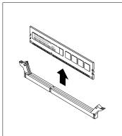
Figure 27. Removing a memory module
