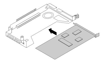
Figure 44. Installing a PCIe card
