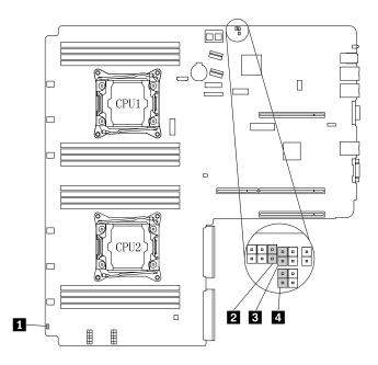
Figure 16. System board jumpers
