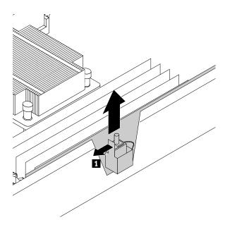
Figure 53. Removing the intrusion switch
