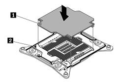
Figure 106. Installing the microprocessor socket cover
