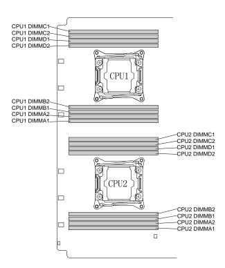
Figure 24. Memory slots on the system board
