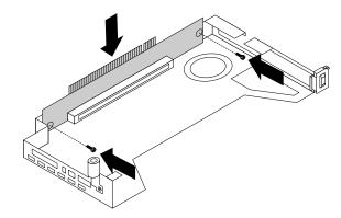
Figure 98. Installing the riser card
