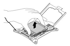
Figure 64. Removing the microprocessor
