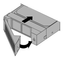
Figure 81. Installing the bracket with the solid-state drive
