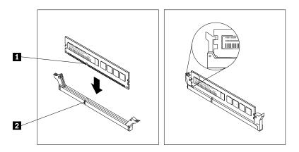
Figure 26. Installing a memory module
