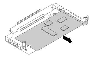
Figure 47. Removing the PCIe card
