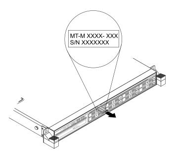
Figure 2. Label on server models with 2.5-inch-drive bays
