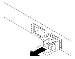
Figure 51. Removing the optical module
