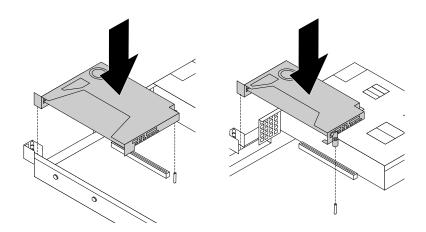
Figure 99. Installing the riser card assembly
