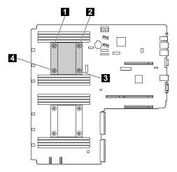
Figure 55. Installing the screws to secure the heat sink
