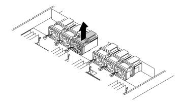
Figure 92. Removing the system fan
