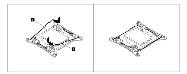
Figure 61. Securing the microprocessor in the socket
