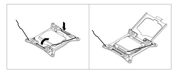
Figure 63. Opening the microprocessor retainer
