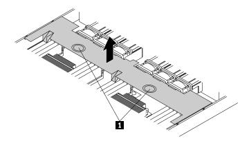
Figure 22. Removing the cooling shroud
