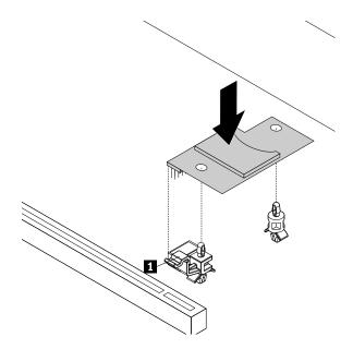
Figure 36. Installing the SD module
