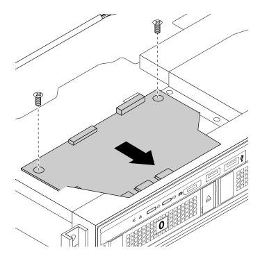
Figure 95. Installing the front panel board
