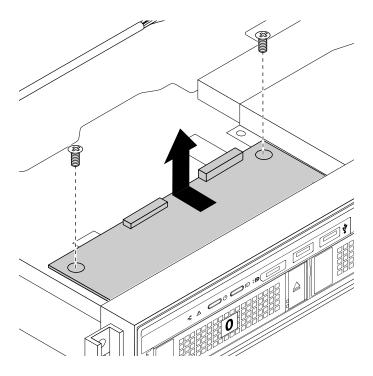
Figure 94. Removing the front panel board
