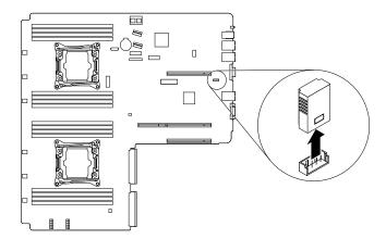
Figure 29. Removing the TSM Premium module
