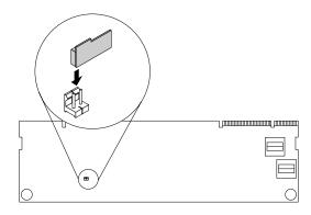
Figure 34. Installing the RAID 500 key
