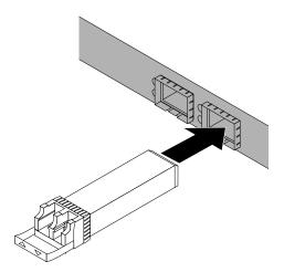
Figure 48. Installing the optical module
