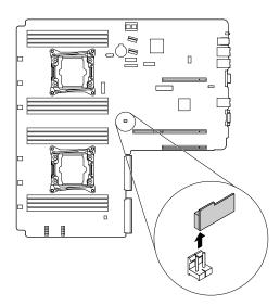
Figure 33. Removing the RAID 110i key
