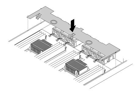
Figure 23. Reinstalling the cooling shroud
