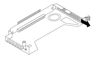
Figure 43. Removing a PCIe slot bracket
