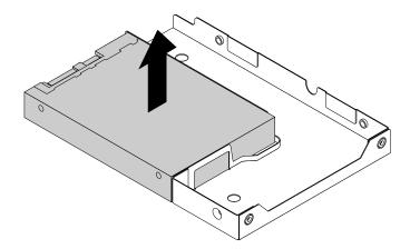
Figure 86. Removing the solid-state drive from the drive adapter
