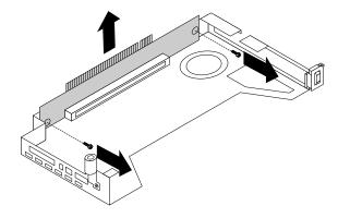
Figure 97. Removing the riser card
