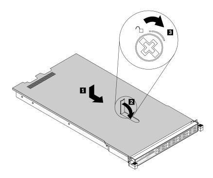
Figure 107. Installing the server cover
