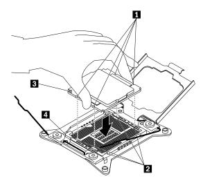
Figure 66. Installing the microprocessor
