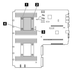
Figure 54. Removing the heat sink
