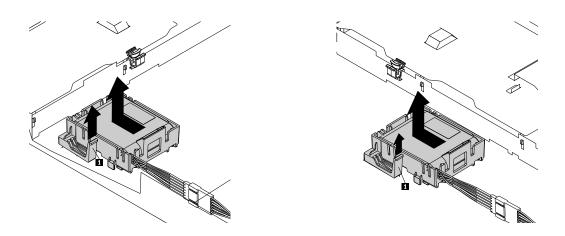
Figure 40. Removing the ThinkServer RAID Super Capacitor Module
