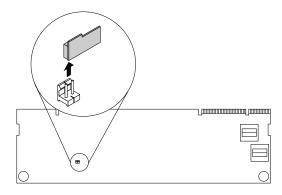
Figure 35. Removing the RAID 500 key
