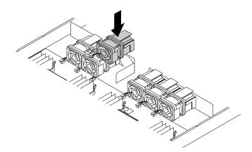
Figure 93. Installing the system fan
