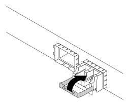
Figure 49. Pivoting the optical module handle to the closed position
