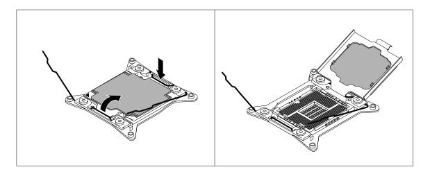
Figure 57. Opening the microprocessor retainer
