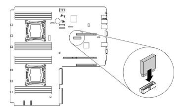
Figure 30. Installing the TPM
