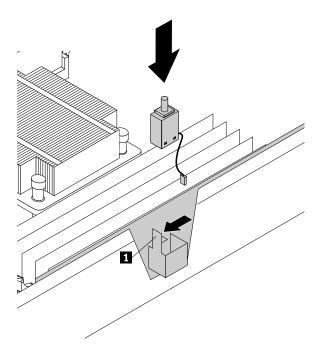
Figure 52. Installing the intrusion switch
