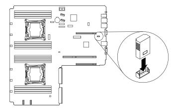
Figure 28. Installing the TSM Premium module
