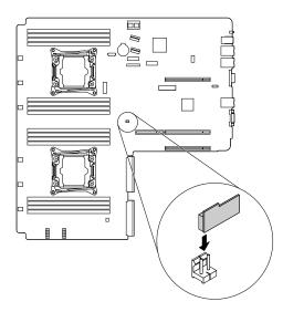
Figure 32. Installing the RAID 110i key
