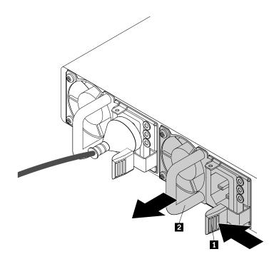
Figure 71. Removing a hot-swap redundant power supply
