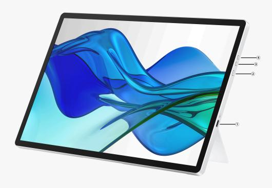
1. USB Type-C<sup>®</sup> (up to 65W USB Power Delivery, Alt Mode DisplayPort<sup>™</sup> 1.2) 2. Power button
