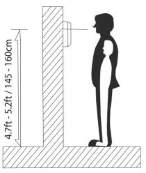
The ideal installation height of the Doorphone is about 4.7ft-5.2ft / 145-160cm from the ground.
