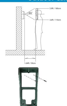
To mount the outdoor camera run the cable from the Doorphone and pull it through the hole you created at the camera mounting point, and then use the four screws to secure the mounting bracket to the wall with the wire inside the bracket so you can connect the camera.
