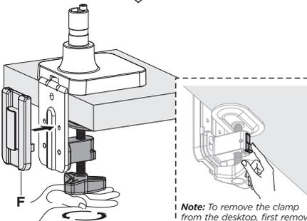
After positioning the monitor arm in the desired location, push up on the clamp knob, then fully tighten the knob.
