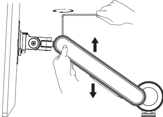
To properly balance the arm with monitors mounted, adjust the spring tension using the supplied Allen Key as follows:
