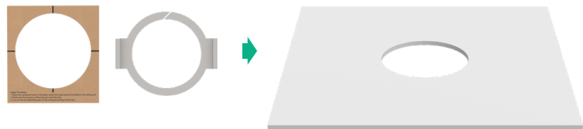
Opening diameter: 200-205mm; Opening depth: 80mm
