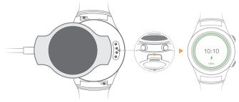
Make sure the charging port is dry and clean before charging to prevent the magnets from being damaged by any moisture.
