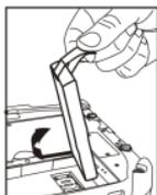
2. Lift the battery using the pull strap and move it aside. Do not disconnect the battery.
